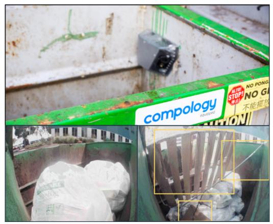
Compology's cameras automatically identify and measure contamination to provide standardized scoring, alerts, and reports to reduce contamination at the source.
