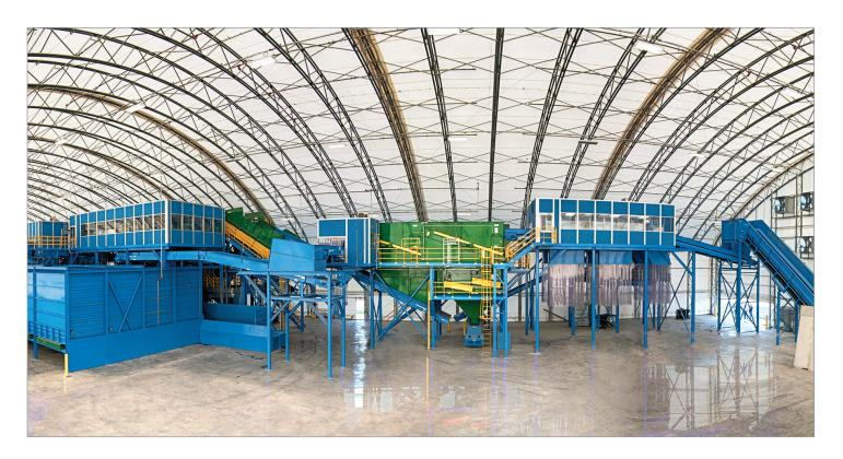
The NRT optical sorter is configured to eject PET containers upward and mixed plastics downward while allowing residue to feed into a middle bin. HDPE is handpicked before the optical sorter.
