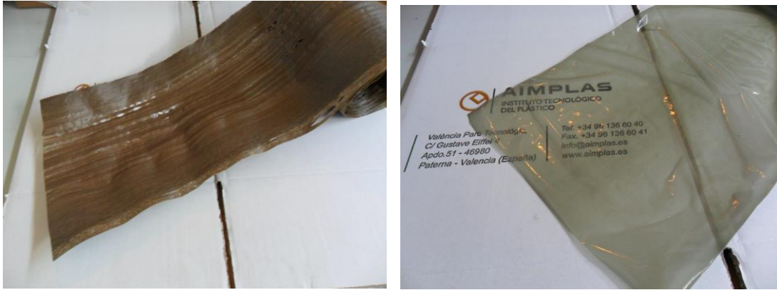
Figure 5. Extruded opaque sheet of thermoplastic material from printed film waste (left) and translucent sheet of granules obtained with the sc-CO 2 extrusion process.
