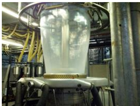
Figure 4. Blown film extrusion from LDPE pellets.
