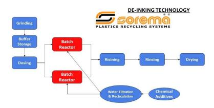
The Sorema "deinking" process is mainly applied to post-industrial waste, but it is also being studied for use in post-consumer waste recycling plants. Very good results have been achieved in numerous applications, but unfortunately, not all types of printing inks are completely removable. For this reason, the pilot plant line in operation at Sorema's RRC "Recycling Research Center", located in Alzate Brianza, has been optimised with the necessary full scale modules for the "deinking".
