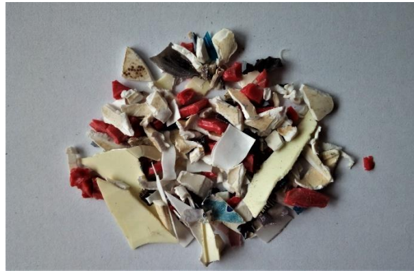
Fig. 1. Mixed stream consisting of materials recovered from marine litter.
