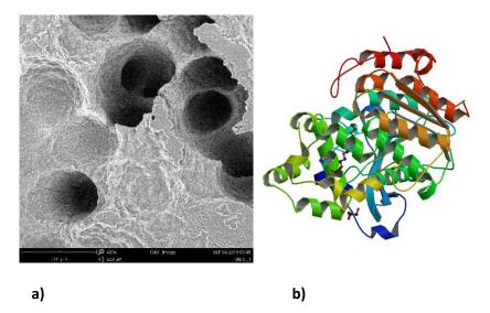
**Figure 1**. a) The surface of a polyurethane film after microbial degradation; b) Three-dimensional structure of the *Candida Antarctica* lipase A enzyme.
