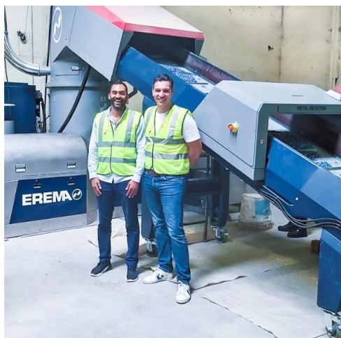
Keiran Smith and Karim Debabe in front of the brand new INTAREMA® 1108 TVEplus® Re grindPro® made by EREMA. The machine processes up to 500 kg/h of HDPE and up to 600 kg/h of PP plastic from household waste to produce recycled pellets.
