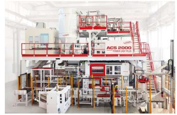
the film thickness has a range from 6 to 25  $\mu$ . Production speed of 850 m/min and mechanical speed up to 1000 m/min. The upgraded technology includes the T-Die Essentia (AMUT branded) with die splitter, movable vacuum box for cleaning without dismantling, jumbo type chill roll unit 1500+450 mm diameter, AD Scan X-Rays thickness control system, the Prowind 4.0 super-fast winder for hand, machine and jumbo rolls without any hydraulic components.
