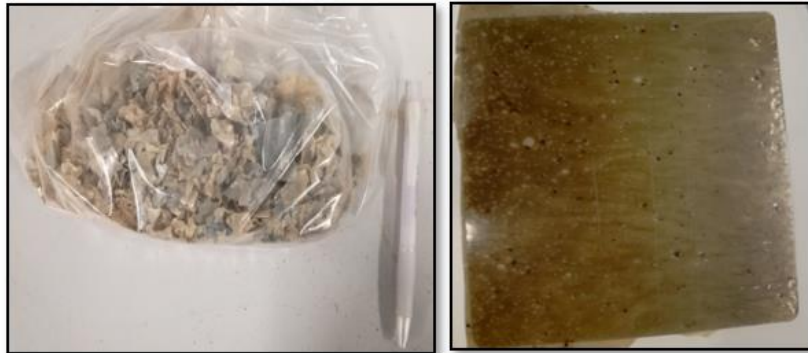
Figure 5. Grinded PET sample and thermoformed sheet.
