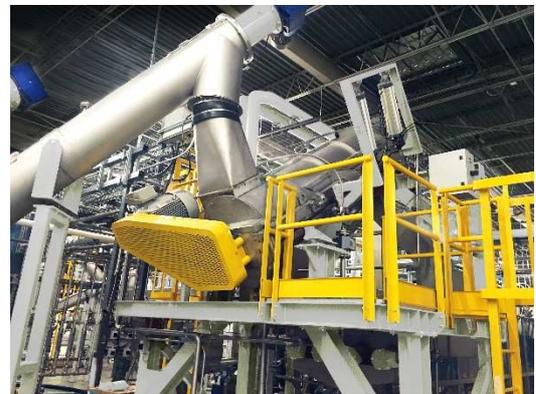
**AMUT has carried out both technology for POAL treatment and washing and the extrusion line to turn the final material into pellets.**
