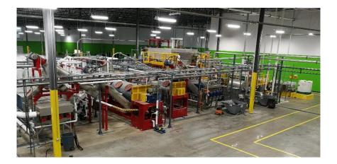
AMUT scope of machinery & technology supplied includes as well, the wet grinding system to turn bottles into flakes, along with two or the AMUT patented Flake Friction Washers, and two of their newest advance technology 'Sink-Float' separation machines, which are able to capture the POLYOLIEFIN caps so that the value of these cleaned caps can also be captured. (See the above photo.)
