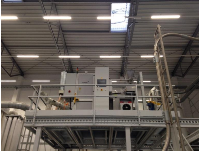
Polysecure Tracer Based Sorting machine within an industrial production environment
