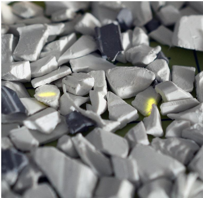
PVC flakes from window profiles marked with fluorescent tracer from Polysecure – fluorescent flakes are separated from non-fluorescent flakes.
