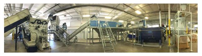
Lindner's washing line. Connected to the single-shaft pre-shredder Micromat Plus is a Floater, a Twister and a Graviter, followed finally by a dryer and air-wash system. © Lindner washTech <<Note to Editor: further images at end of release>>
