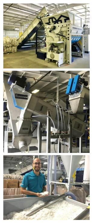
The single-shaft Micromat Plus 2000 pre-shredder from Lindner is fed by conveyor belt with the nonreturnable HDPE milk containers compressed into bales.
