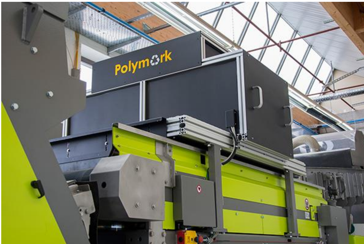
The Polymark sorting machine made by Sesotec with Polymark detector unit for the detection of UV fluorescence markers on PET bottles. (Photo: Sesotec GmbH)
