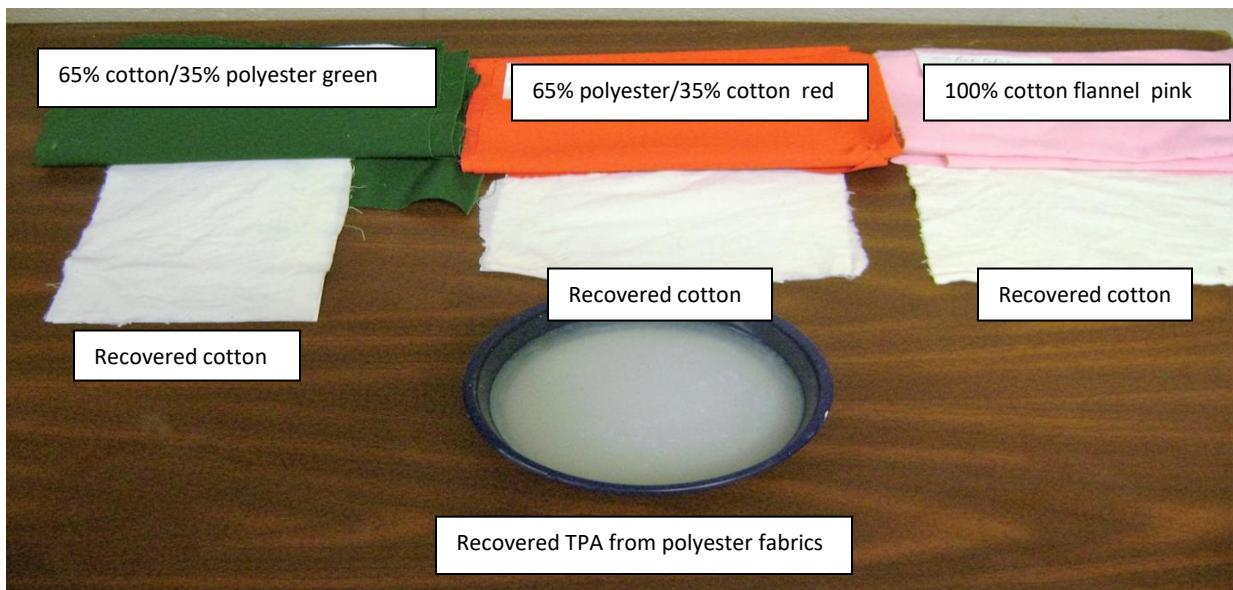
The dyes in these fabrics were completely removed along with PET within 20 minutes in the reagent at temperatures of 100-110° C. Samples were retested to confirm that PET was completely removed. The Terephthalic acid resulting from the depolymerization of PET is shown below in the dish.
