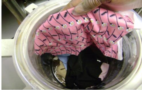
Picture 2 – Fabrics are placed into the reactor containing preheated reagent
