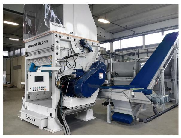
Used as a pre-shredder, the new Lindner Micromat WS wet shredder is the first step in washing systems for post-consumer plastic scrap. Together with another two new downstream systems, the Rafter Pre-washer and the Loop Dryer, it is part of the innovative plastics shredding and washing system solution which the Lindner Group from Austria will be premiering at K 2016. © Lindner Recyclingtech
