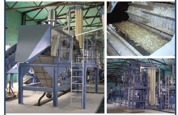
Wet Granulators • Friction Washers • Separation Tanks Hot Wash Systems • Hydro Cyclones • Thermal Dryers Mechanical Dryers • PVC Label Removers
