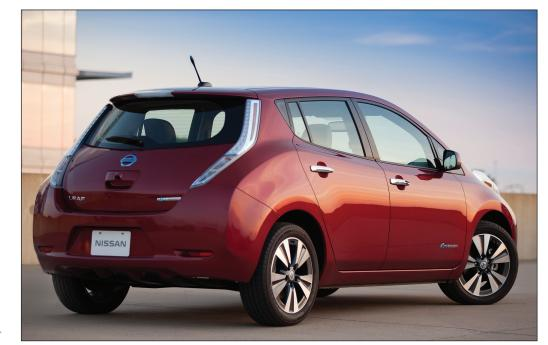
made using recycled content. The 2015 Nissan Leaf weighs roughly 3,200 pounds and uses 800 pounds worth of recycled materials. The compact hatchback's seats, for instance, utilize a fabric made from reclaimed PET plastic, and the car's center console leverages plastic that comes from end-of-life household appliances.
