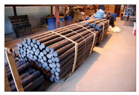
Fence stock is shaped and cut to make uniformly-fitting posts and rails. Standard woodworking tools can be used to easily cut, staple or screw into the plastic fencing and insulators are not required for electric fence installation. Plastic posts are virtually solid and do not require timber or metal inserts. One two-rail section of fencing is made from the equivalent of 525 gallon-sized HDPE milk jugs.
