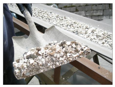
mixture contained 25 percent recycled ceramic material and 75 percent asphalt and gravel. All told, 400 porcelain toilets were used to repave city sidewalks as part of the Meader Kansas Ellis Trail Project. The cost of making and laying down the alternative concrete was on par with traditional methods and came in at \$850,000, along with saving landfill space. Freeman told *Resource Recycling* poticrete is "just as good as crushed rock," but slightly lighter.
