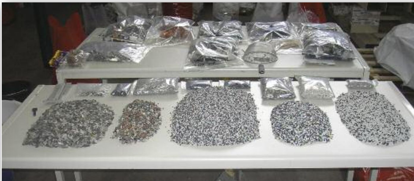
Samples of dirty and cleaned mixed plastics from obsolete electronics.
