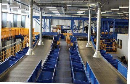
stream processing. To help alleviate this issue, our new facility incorporates 16 plastic bag collection points at pre-sort and post-sort stations." The MRF will also include ample pre-sort areas to help deal with contamination that stems from materials coming from some public drop-off locations.
