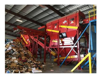
incorporated Right Away Disposal's existing sort lines, conveyors, and a baler with new CP disc screens in order to automate the system, process a higher throughput, and recover more commodities.
